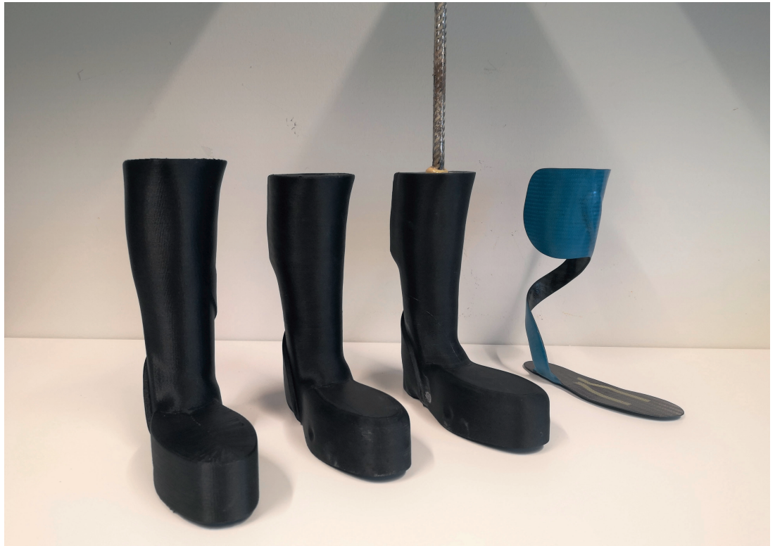
3D-printed laminating standard for the production of CFRP orthoses. © Adviva
